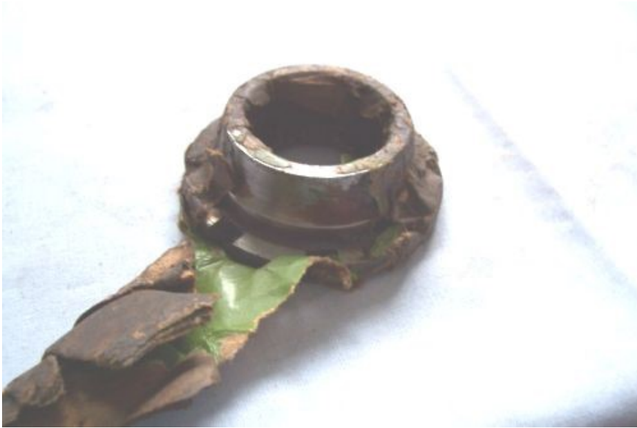
Clutch Spring Retaining Nut Part Number 15-4312
