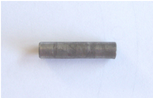
Clutch Operating Lever Thrust Pin 25-4251 and Nut 27-4411
