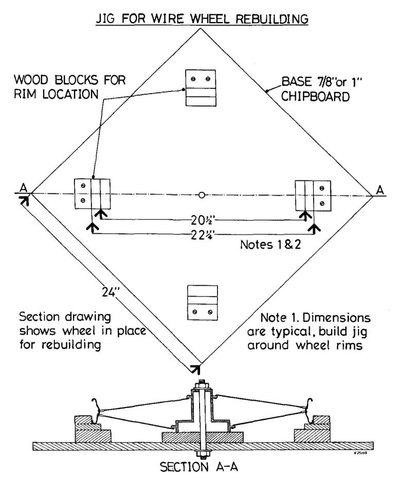
Note 2. Dimensions are for 24"x 24" B.E. tyre wheels & 27x2.75" WIRE EDGE tyre wheels
